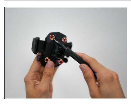
Remove four 5.0 mm screws from the backing panel of the phone holder using the Oval shape screwhead. Push out wing panels to release the mechanism, and remove the screws and holder from the backing panel.
