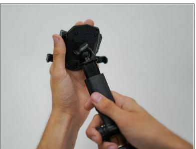
• With moderate to heavy force, apply pressure to the ball joint into the socket.
