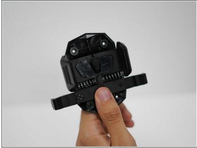
Insert two new 2.6 cm springs as you would batteries to a tv remote. Be cautious as to keep the chassis in place during this process.
