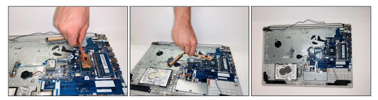
• Gently lift and remove the heat sink and set it aside.
