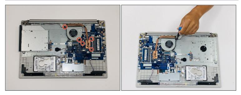
• Remove five 7mm Phillips #00 screws from the cooling fan.
