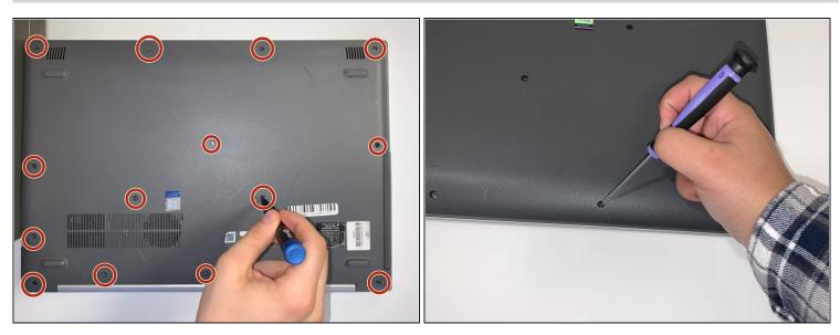
• Remove fourteen 7mm Phillips #00 screws from the back panel.
