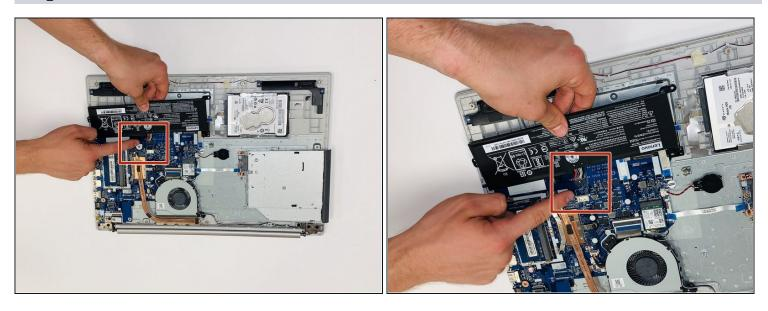
• Pinch the connecting cord with one hand and pry the battery connector with the other hand, while gently pulling the connector straight out and towards the bottom edge of the base.
