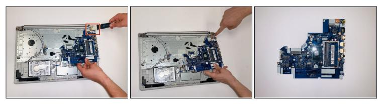
• Using a Jimmy, gently pry the motherboard from under the corner screw holder with one hand and pull the motherboard out with the other.
