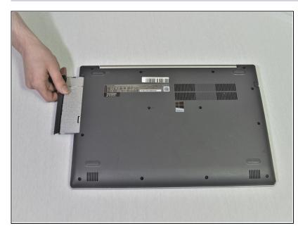
• Carefully remove the optical drive by pulling the bezel away from the laptop.
