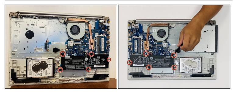
• Remove five 7mm Phillips #0 screws from the battery holder.
