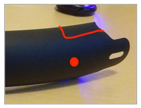
You need to cut both sides of the mudguard so it can fit between the chain stays, and drill a new hole to attach to the bottom of the frame.
