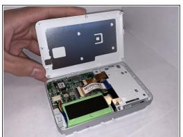
• Flip the LifePrint 2x3 upside down. Using a plastic opening pick, separate the bottom cover from the device and remove it.
