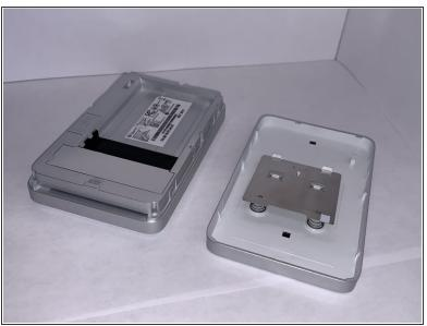
Orient the LifePrint 2x3 so that the top of the device is facing upwards. Slide the top cover toward the far side of the device and remove it.
