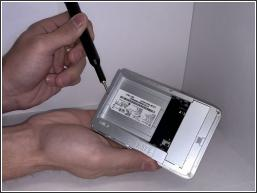
Remove the six 5.24 mm screws located around the edges of the device using a Phillips #00 Screwdriver.
