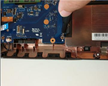
Unscrew eighteen 5.8 mm screws from the motherboard with a Phillips #00 screwdriver.
