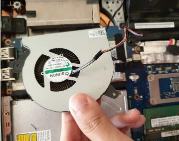
With your hands, carefully lift the left fan and unlatch the fan from the motherboard.
