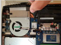
Unscrew one 3mm Philips #00 screw on the wireless card.
