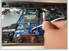
Using an ESD safe tool, detach all 3 ribbon cables. To do so, lift up the cable up and out.
