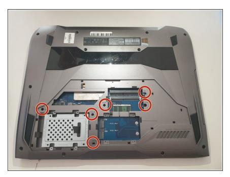
Using the Phillips #00 screwdriver, remove the six 5.2 mm screws under the service cover.
