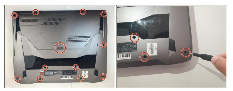
• Using a Phillips #0 screwdriver, remove all twelve 5.2mm screws on the back of the laptop.
