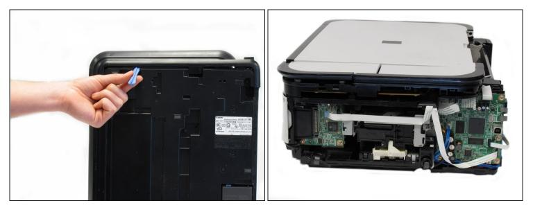
• Use the plastic opening tool to loosen the side panel from the bottom of the printer.
