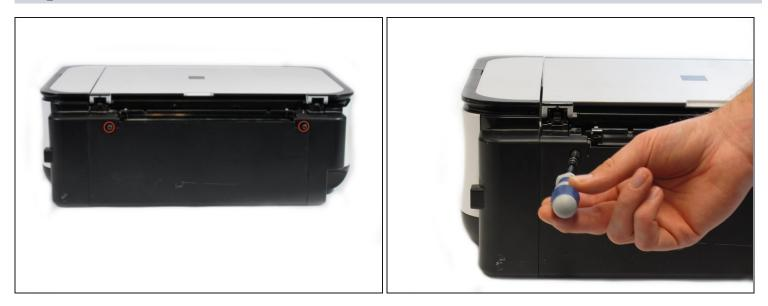
• Remove the two 7.9 mm screws using a Phillips #1 screwdriver.
