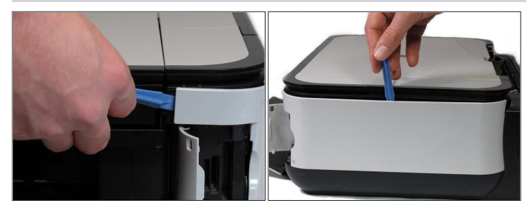
• Pry open the side cover with the plastic opening tool.
