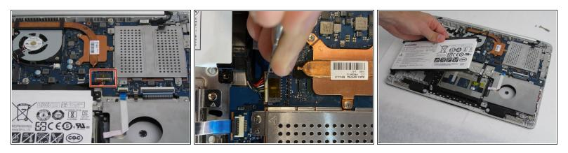
• Use a spudger to pry the battery connecting cable from the laptop and remove the battery.
