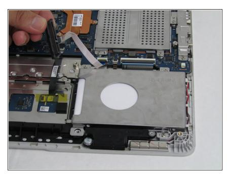
Remove the connection cable from the hard drive.
