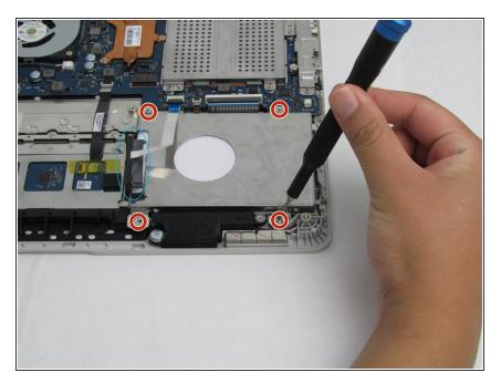
• Use a Phillips #00 to remove four screws from the hard drive cradle.
