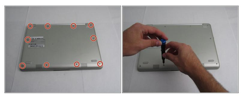
Use a Phillips #00 screwdriver to remove the four 6.5mm screws and the six 4.5mm screws that secure the back plate.
