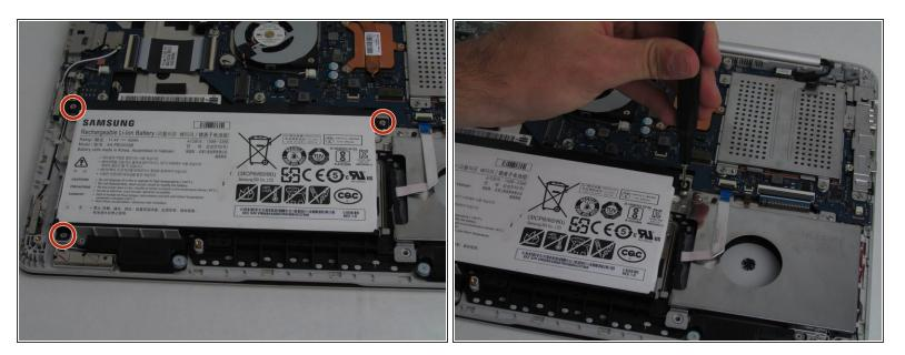
Use a Phillips #00 screwdriver to remove the three 4.5 mm screws holding the battery in place.
