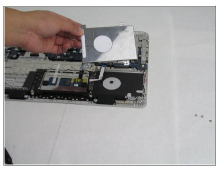
• Pull the hard drive away from the cradle and remove it from the device.
