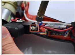
• Desolder the wires soldered to the trigger.
