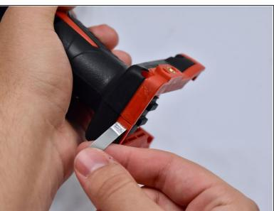
Peel back the sticker at the bottom of the drill handle.
