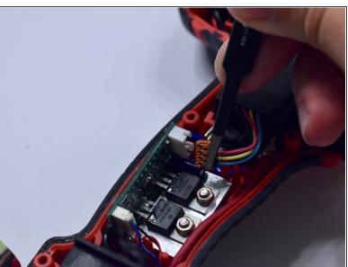
Unplug the 4-pin connector, using the tweezers, from the circuit board.
