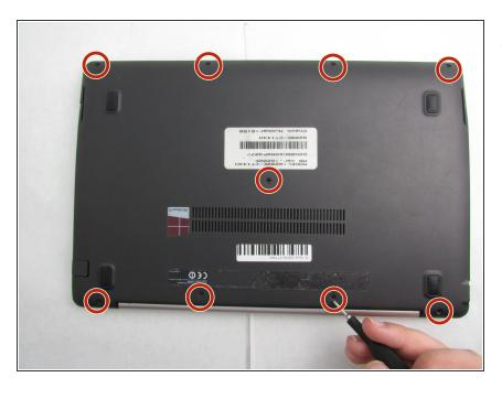
Remove the 9 screws holding the cover in place by taking a Phillips #00 Screwdriver and turning it counterclockwise.
