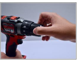
Rotate the chuck counterclockwise as far as possible to loosen from the base.
