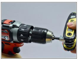
Rotate the Allen wrench counterclockwise to remove the chuck.
