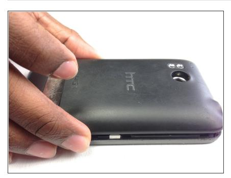
• Lift and remove the rear panel.
