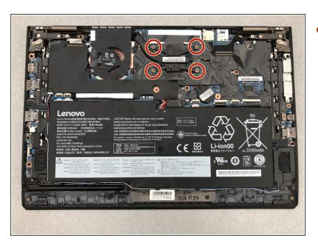
Remove four 4.5mm Phillips #1 screws from the corners of the heat sink.
