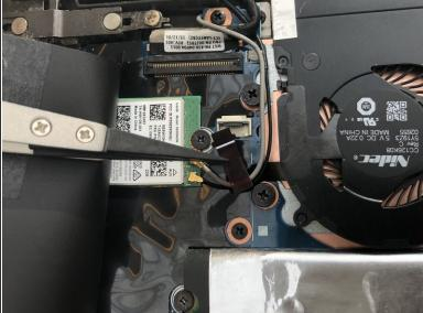
Using tweezers, pull the plastic strip out.
