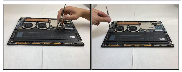
• Use the nylon <u>tweezers</u> to remove the interconnect pins from each of the circuit boards.
