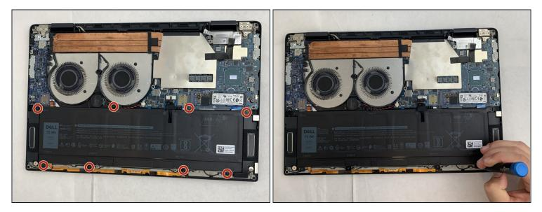
• Use the Phillips #0 screwdriver to remove all eight 6.4mm screws from the battery
