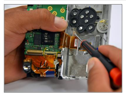
• Remove the 4mm Phillips #00 screw from above the ribbon.
