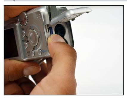
• Press on and release the memory card to eject it.
