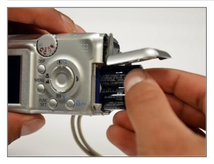
• Tilt the camera slightly to allow the batteries to fall out.
