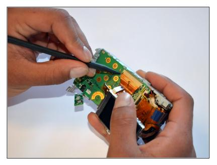
• Using a spudger, lift the grey tabs to allow the ribbon to slide out.
