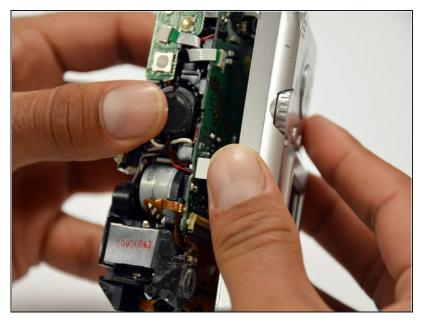
• Remove the back case of the camera by pulling from the top.
