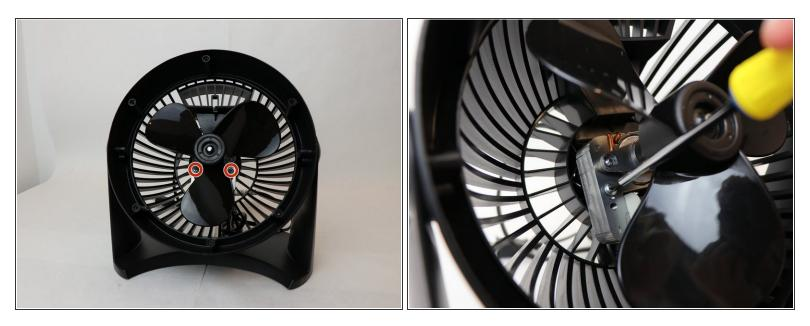
Remove the two 36mm screws on the metal plate behind the blades using the Phillips #1 screwdriver.
