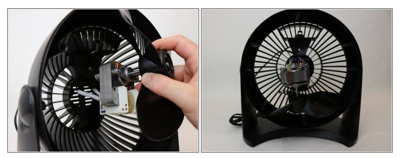
Carefully pull the motor forward out of its resting position and tilt it forward revealing the back of the motor.
