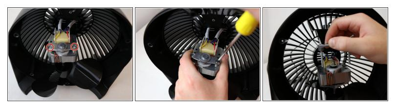
Using the Phillips #1 screwdriver, remove the two 37mm screws on the back of the motor.
