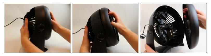
• Pry apart the blade cover from the body of the fan to access the inside.
