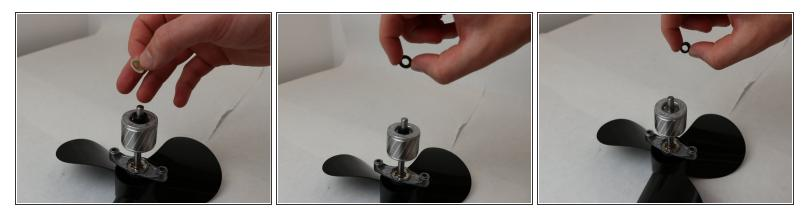
• Remove the felt washer, metal washer, and the rubber stopper from the axle.
