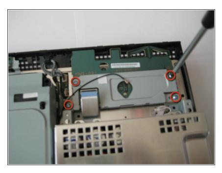
Remove the four Philips #2 screws from the top of the wireless assembly.
