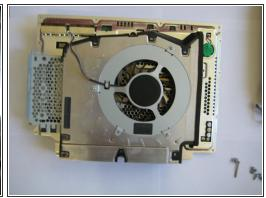
Remove the fan power connector.
