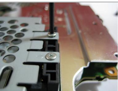
Remove the 2 Phillips #0 screws from the hard drive enclosure.
