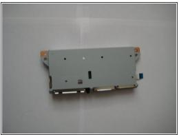
To remove the plastic card reader, locate its two locking plastic tabs that hold the card reader to the shell, spread them, and lift the card reader off of the shell.
