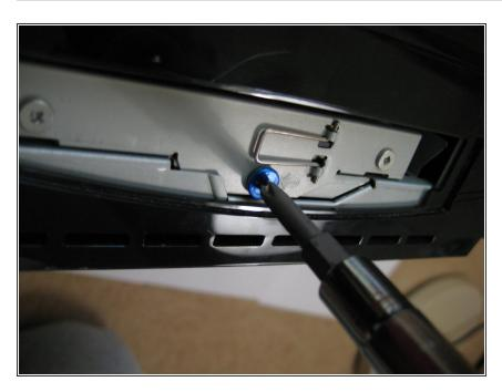
Use the Phillips screwdriver #1 to remove the blue screw.
