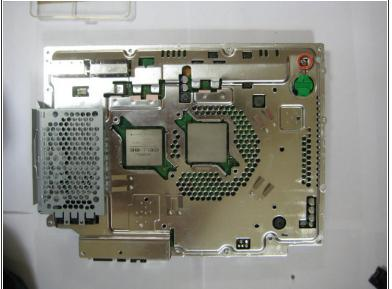
To expose the mainboard, remove the watch battery from the mainboard.
