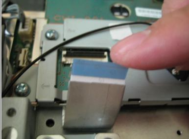
Remove the flat ribbon cable from the wireless assembly.
