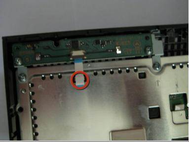
Remove the ribbon cable attaching the on/off and eject switch circuit board to the main board.
