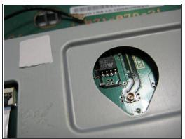
Working on the main unit, lift up on and disconnect the black RF wire from the wireless assembly using a spudger.
