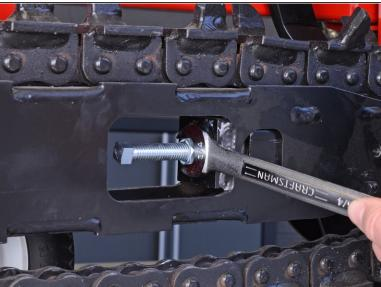
After the chain is properly tensioned, use a 3/4 inch open-end wrench to tighten the adjuster screw locknut.
