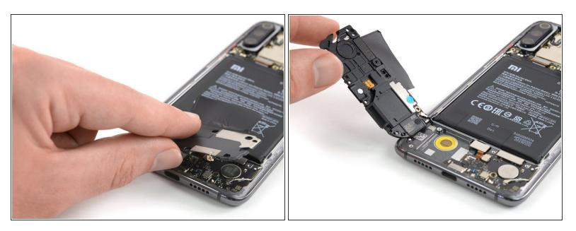
There is still an antenna cable connected to the back of the unit.
