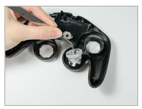
Use tweezers to grab the center peg of the directional pad and lift it out of its socket.
