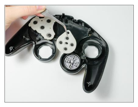
Remove the rubber backing with tweezers.
