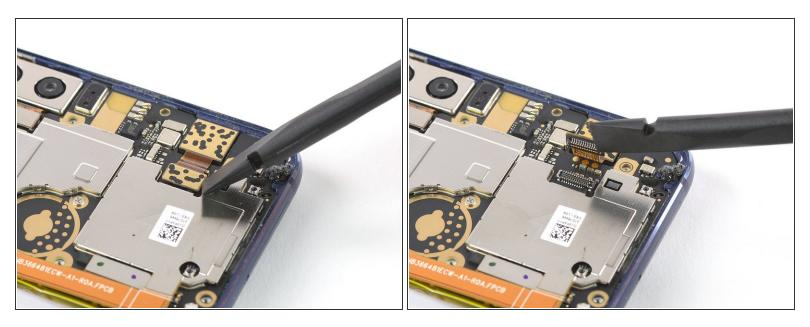
• Use a spudger to pry up and disconnect the front camera flex cable from its motherboard socket.
