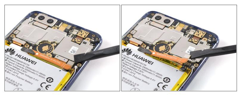
Use a spudger to pry up and disconnect the battery flex cable.
