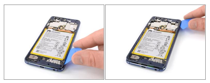
Repeat the procedure on the right edge of the phone to cut the adhesive underneath the midframe bezel.
