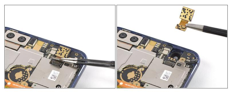
• Use a pair of tweezers to carefully lift the front camera out of its recess and remove it.
