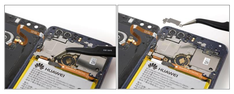
Use a pair of tweezers to remove the metal bracket that sits on top of the fingerprint and display flex connectors.
