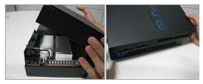
• Put the console in the normal horizontal position, and pull the top cover from back to front.
