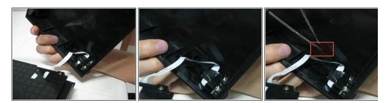
⚠ This model has a flat cable to the reset and eject button. Take extreme caution to not destroy it.
