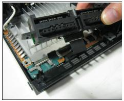
• Remove the two screws with a Philips "0" screwdriver to deatach the controller port.
