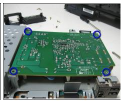
• This is the power source board. remove the 4 screws where I marked in blue.
