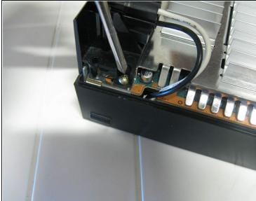
Here we remove the screws from the cooler and the main power switch
