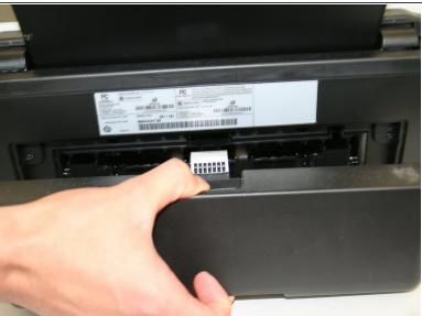
• Check the duplex unit, located at the rear of the printer, for any paper obstruction. Pinch the top button to remove the unit.
