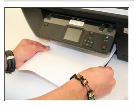
Check the front slot, which is located underneath the LED display. If there is any paper, remove it.
