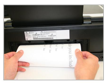
If there is any paper stuck inside, remove it. If not, snap the unit back onto the printer.
