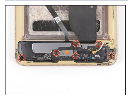
Remove the six 3.4 mm Phillips screws holding the loudspeaker in place.
