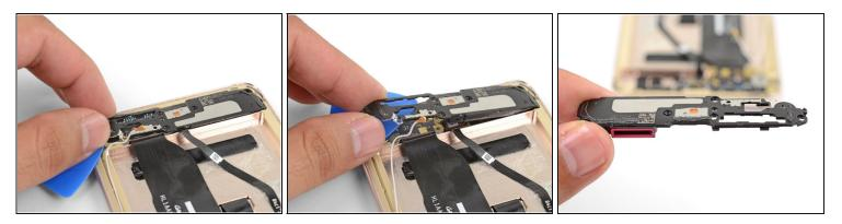
• Grasp the loosened edge of the loudspeaker and gently pull the assembly away from the bottom edge of the phone.
