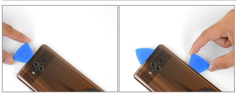
• Continue heating and slicing through the remaining edges, leaving opening picks in the seams to prevent the adhesive from re-sealing.
