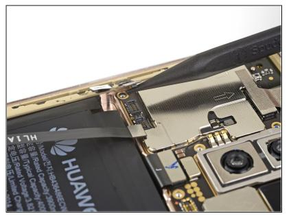
• Use the point of a spudger to pry up and disconnect the button connector from its motherboard socket.
