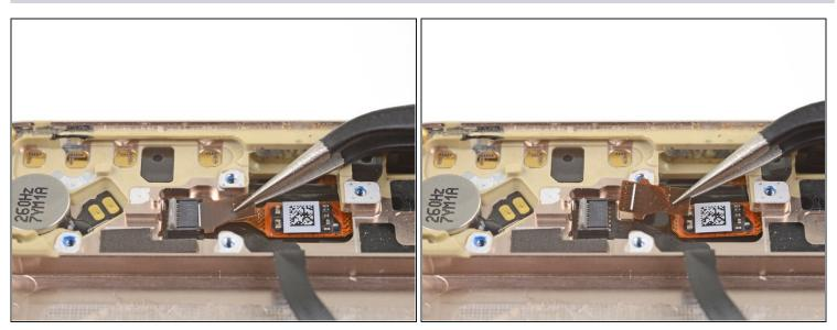
• Use tweezers to grasp the cable's brown pull tab and pull the cable out of the socket.
