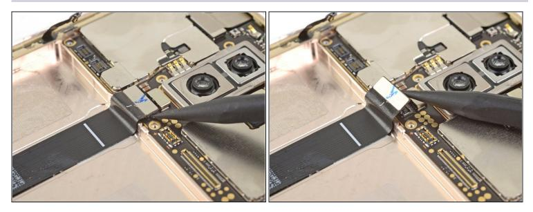
• Use the point of a spudger to pry up and disconnect the display cable from its motherboard socket.
