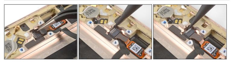
• Use tweezers to peel the tape covering the fingerprint sensor cable connector near the bottom edge of the phone.
