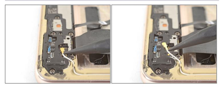
• Use the point of a spudger to pry up and disconnect the white antenna cable from the bottom of the phone.
