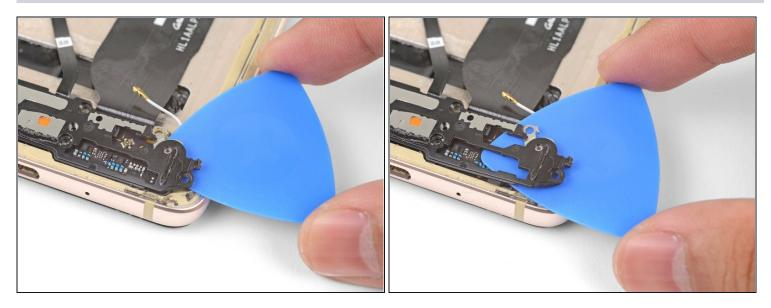
(i) The loudspeaker is still held in place by adhesive and clips.
