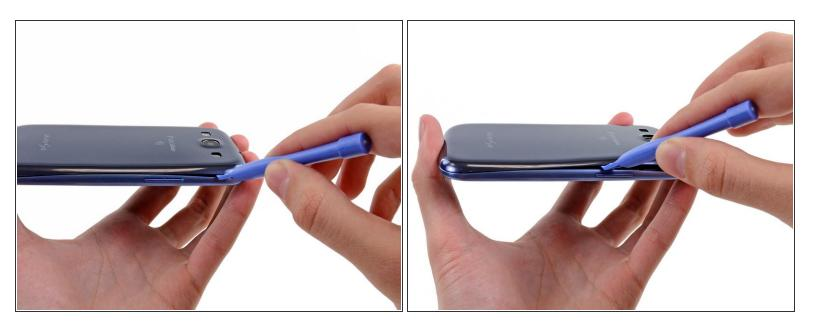
Continue to move the plastic opening tool around the perimeter of the top left corner, gently prying up along the rear case.
