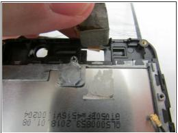
There will be a thin flat cable at the top of the screen in which you need to carefully peel back.
