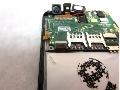
Desolder the gold ribbon that is connected to the motherboard at the bottom left corner.
