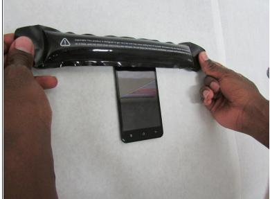
Apply the heated iOpener to all sides of the screen (left, right, top, and bottom) for 90 seconds (or more if necessary) to soften the adhesive.
