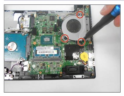
• Using a #0 Phillips screwdriver, remove the three 3mm screws around the perimeter of the fan.
