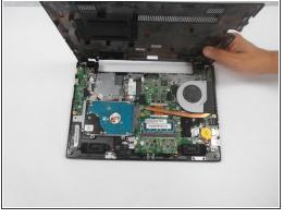
Slowly begin working your plastic opening tool along the panel to undo the latches around the laptop.
