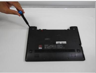
Using the #0 Phillips screwdriver, remove the nine 4mm screws on the back panel.
