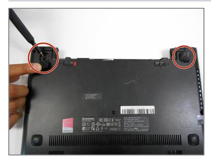
• Gently pull the two rubber feet closest to battery away from the device. Using a #0 Phillips screwdriver, remove the 5mm screw under each rubber foot.
