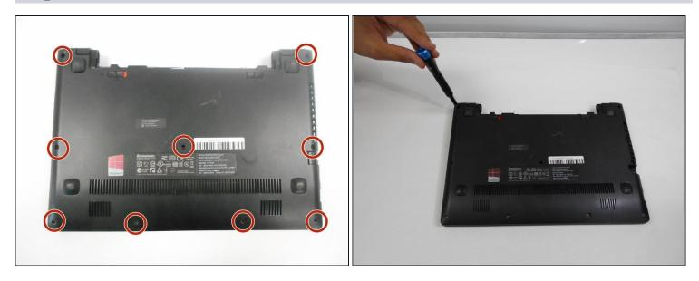
• Using the #0 Phillips screwdriver, remove the nine 4mm screws on the back panel.
