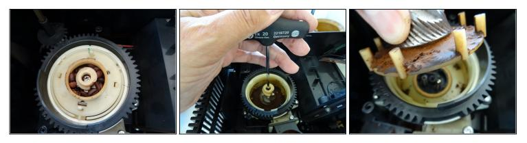
• Now the grinder is free. Again take a picture, then pull out the axis of the adjuster with moderate force.
