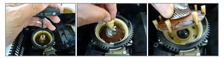
$\triangle$  In the next step be very careful not to loose these three springs, balls and cartridges.
