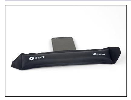
Apply a heated iOpener to the bottom edge of the phone for a minute to loosen the adhesive holding the charging assembly in place.
