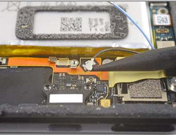
• Use the point of a spudger to pry up and disconnect the black antenna cable from its socket near the USB-C port.
