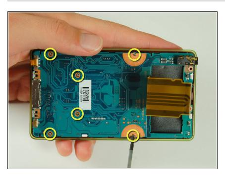
With a Philips #00 screwdriver, remove the six 4.2 mm screws that attach the logic board to the front plate.
