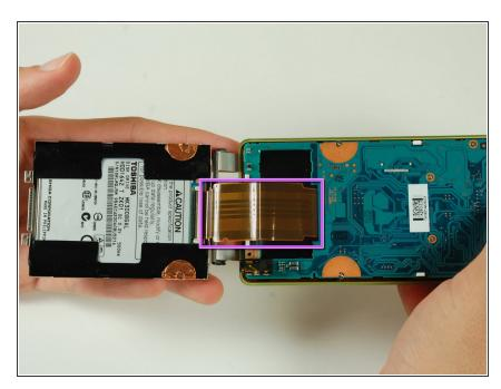
Flip the hard drive over the top to expose the ribbon cable.
