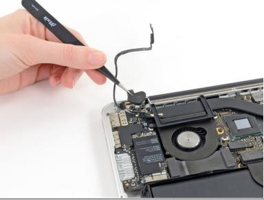
Use a pair of tweezers to lift the rubber hinge covers up off the right and left display hinges.
