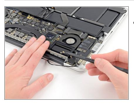
Move the antenna cables aside, clear of the AirPort board.
