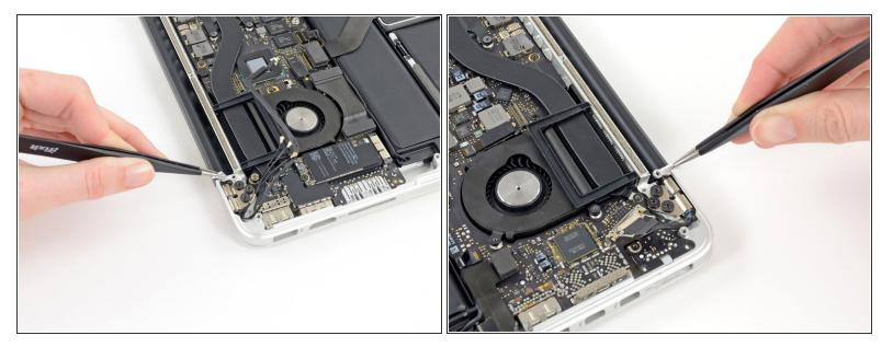
• Use a pair of tweezers to lift aluminum hinge brackets off the right and left display hinges.
