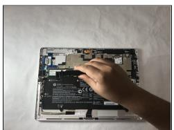
• Remove two 2.7 mm screws using the Phillips #0 screwdriver.
