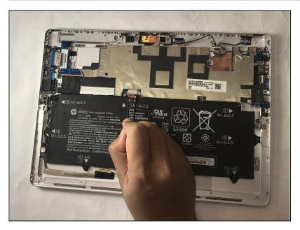
Unplug the battery wire attached to the motherboard using tweezers.
