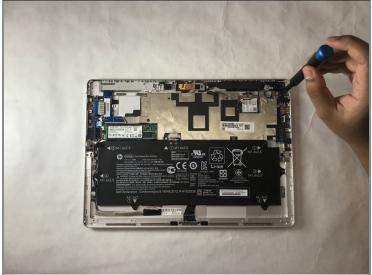
• Unplug the speaker wire attached to the motherboard.
