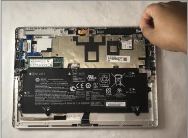
• Detach the right speaker cables from the motherboard using tweezers.
