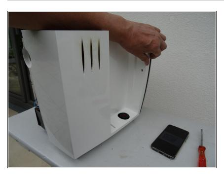
Pull the left side panel slightly towards the back and remove it. Follow the steps in reverse order to reassemble your device.
