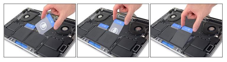
• Retrieve your second plastic card and repeat the previous step to separate the remaining center battery cell.
