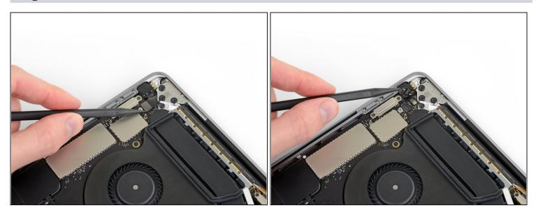
• Disconnect the headphone jack cable by prying its connector straight up from the logic board.
