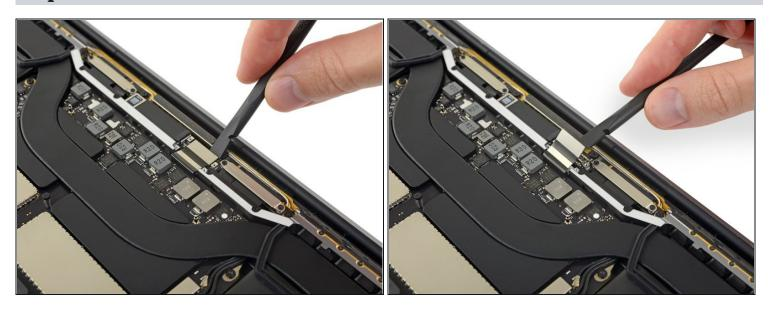
• Pry straight up with your spudger to disconnect the display board flex cable.
