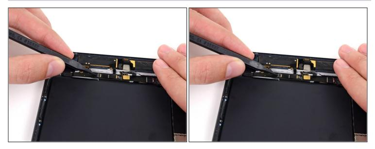
• Use the tip of a spudger to gently lift the tab on the top left antenna ribbon cable's ZIF connector.
