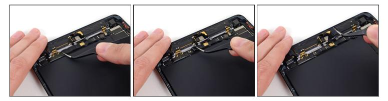
• Use tweezers to peel and remove the long thin black tape covering the top of the headphone jack cable.
