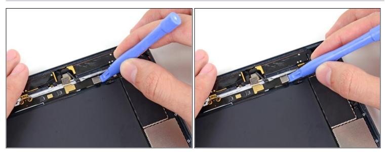
• Use a plastic opening tool to pry the headphone cable's connector up from the logic board.
