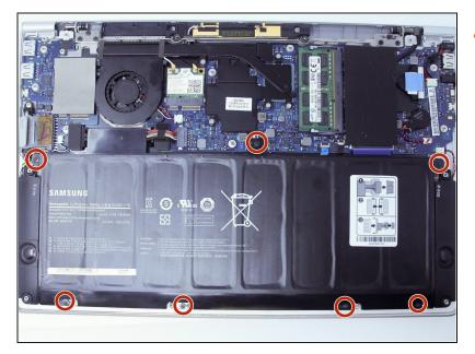
Remove the seven 0.5 mm Phillips #00 screws.
