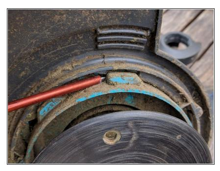
Remove black protection against grass. Do that by rotating it. Rotation is blocked at two places that you can press with a thin screwdriver.
