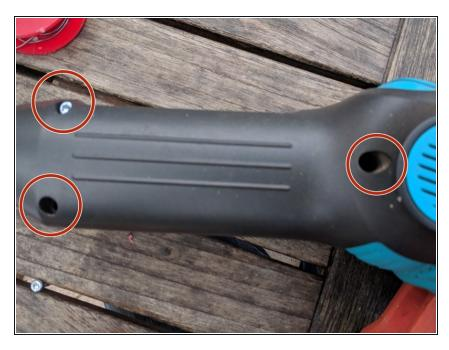
• Unscrew the three visible screws, surrounded in red in picture.
