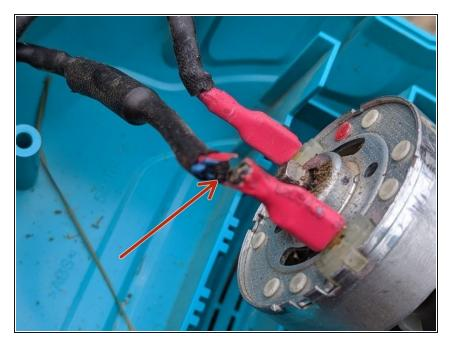
Clean, fix and re-protect damaged connector.
