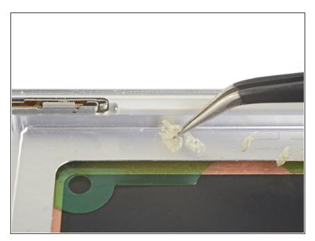
Remove any remaining adhesive from the phone frame, and clean the glued areas with isopropyl alcohol and a lint-free cloth.
