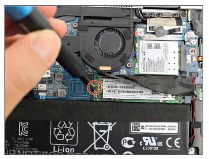
Remove the 2.4 mm screw using a Phillips #00 screwdriver.
