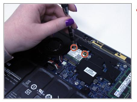
Remove the two 2.5 mm Phillips #00 screws.
