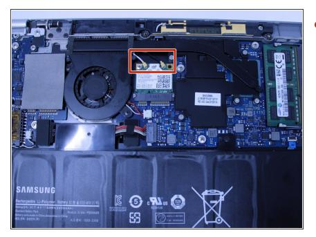
Remove the two wires connected to the WiFi card using a nylon spudger.
