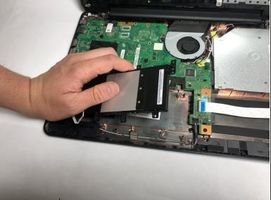
Lift up battery and remove it from the device.
