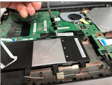
Remove the four 4 mm Phillips #0 screws securing the battery.
