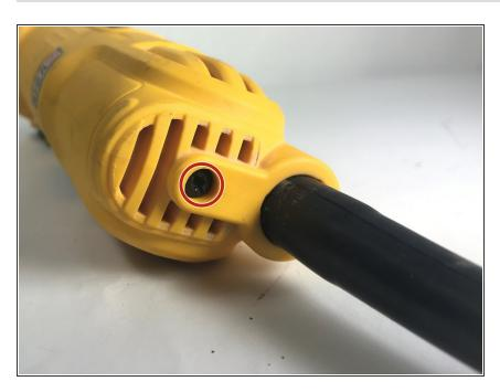
Turn to the bottom of the device and remove the 5/8" (17mm) T15 Torx screw.
