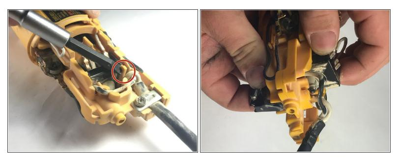
Pull back the yellow tab holding the housing in place using a nylon spudger. Carefully pull the housing out of the casing.
