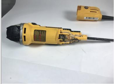
Remove bottom casing by separating the end handle away from the main casing.
