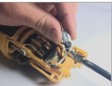
Remove the 1/2" (13mm) Phillips #2 screw holding the power cable to the device. This will free up the metal clamp holding the cable in place.
