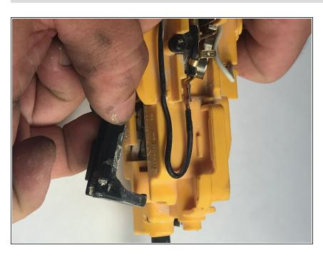
Flip the grinder over and disconnect the plastic switch mechanism from the cable housing.
