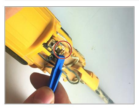
Using an iFixit opening tool, remove the female terminal connecting the carbon brush wire to the male terminal.
