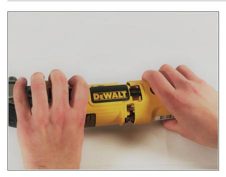
Remove outer casing by pulling the end handle away from the field case.
