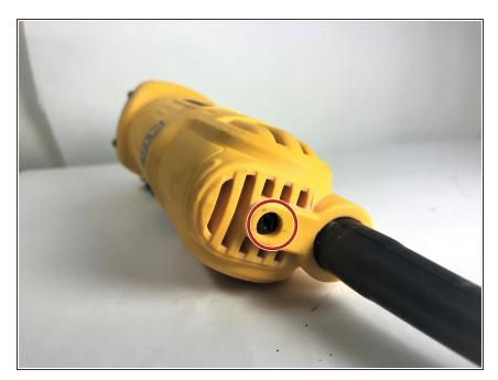
Turn to the bottom of the device and remove the 5/8" (17mm) screw shown using a T15 Torx Screwdriver.
