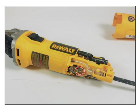
Locate the brush springs on either side of the device.
