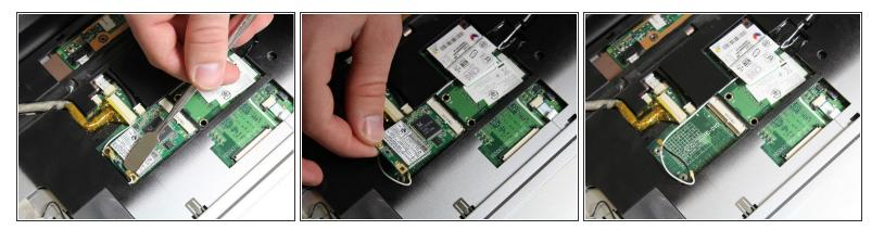
After removing the keyboard, gently pry upwards on the gold contacts holding the white and black WiFi antennae wires using a rubber spudger to release them from the card. Then, simply pull upwards and out to remove the card.
