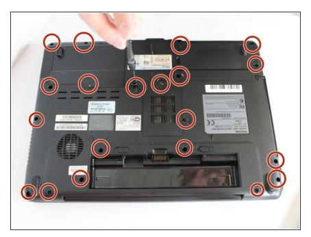
Remove all the 3mm long screws on the underside of the laptop.
