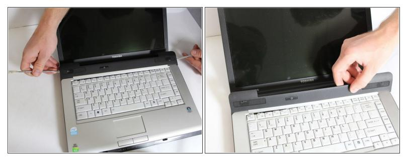
• Remove the black plastic bezel above the keyboard by prying upwards with a flat object.
