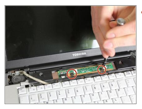
Remove the two Phillips #00 2mm long screws located under the bezel that hold the keyboard to the chassis.
