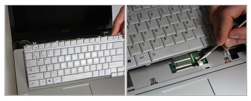
• Lift the top of the keyboard and press the pins retaining the keyboard ribbon cable towards the screen with a rubber spudger to release the keyboard from the laptop. Set the keyboard aside.
