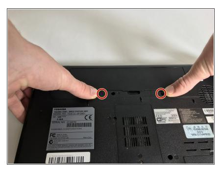
Push the two plastic tabs retaining the battery into the chassis to each respective side. This will push the battery up slightly and release it from the bottom of the notebook.
