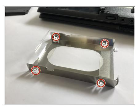
The hard drive will be held in the hard drive caddy by four 1.5mm Phillips PH00 screws. Remove these screws to remove the old drive and install a new hard drive or solid state drive. To reassemble your device, follow these instructions in reverse order.
