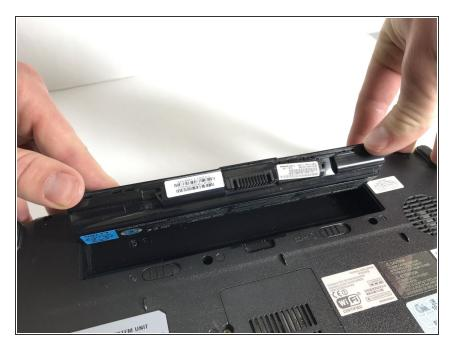
Using a finger or small prying device, pull the battery upwards from the recessed area. Then, simply pull the battery out of the notebook and gently set it aside.
