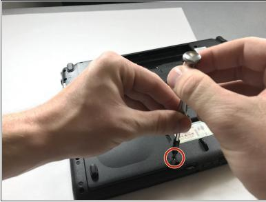
Remove the two 3mm Phillips #00 screws holding the hard drive bay cover in place.
