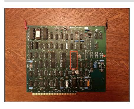
Remove the chip marked 8530 at location 9D.
