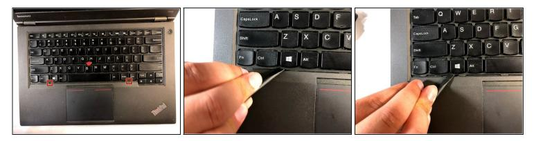
• Using the spudger, move the plastic protector by pressing it down and forward in order to uncover the screws.
